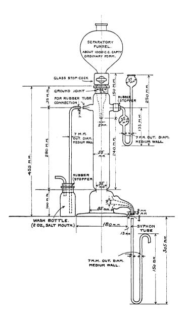
table top allowing the siphon tube to be carried underneath, whence it can discharge into any convenient receptacle.
